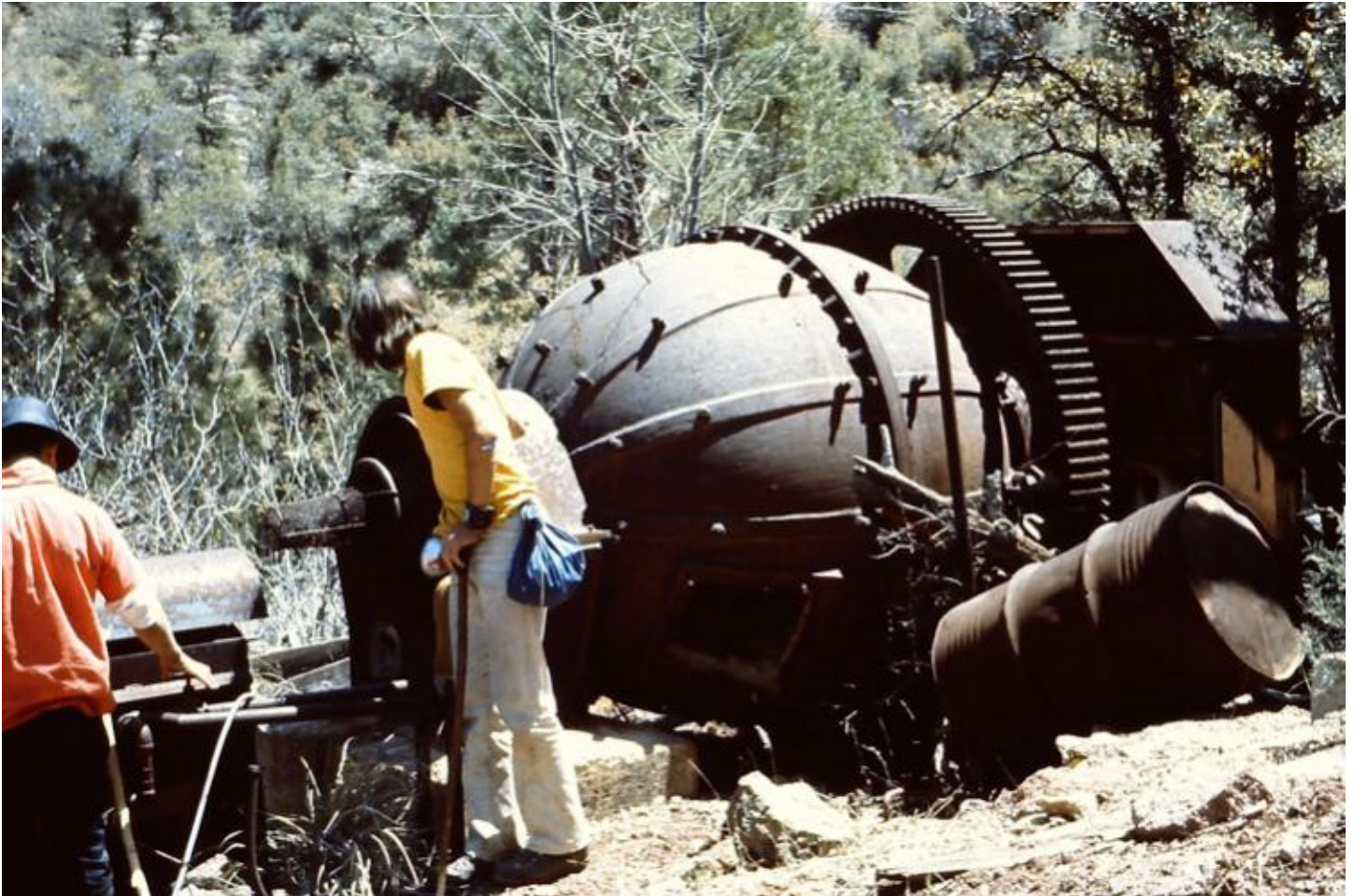
The remains of an abandoned ball mill in Arizona. The rest of the mill has fallen into ruins.
