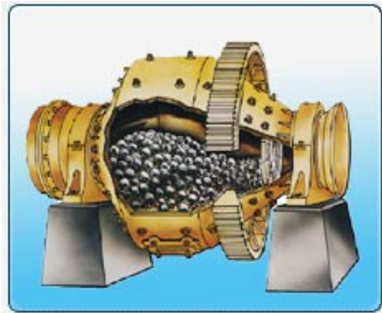
A CUT-AWAY VIEW OF A BALL MILL. THE ORE-CRUSHING IRON BALLS ARE SEEN INSIDE.
