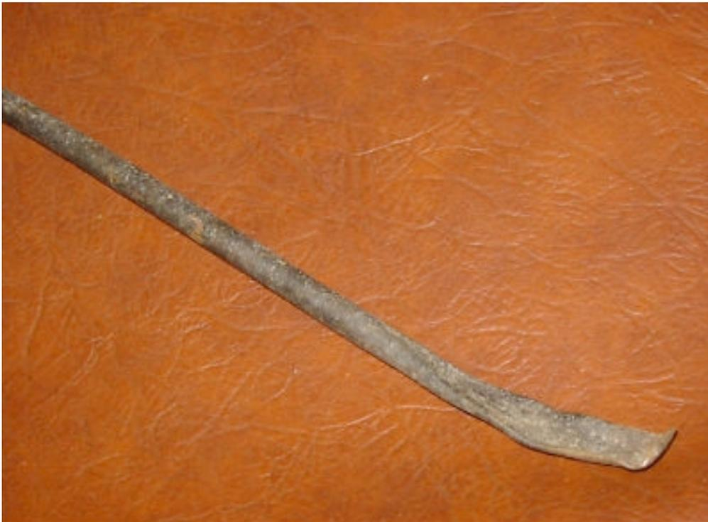
*An antique metal cleaning spoon used to clean the dust and debris out of a drilled hole so the sticks of powder could be tamped down.*
